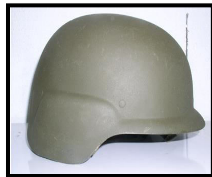
Figure 12 Light weight natural composites military Helmet
