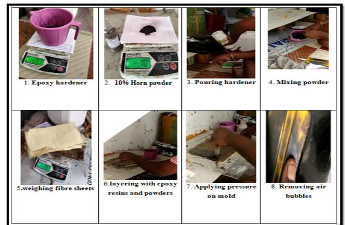
Figure 19 Complete sequential process for fabrication
