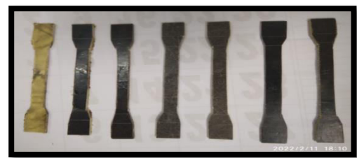
Figure 20 Tensile test specimens
