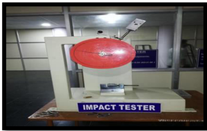
Figure 22 Impact machine for impact testing
